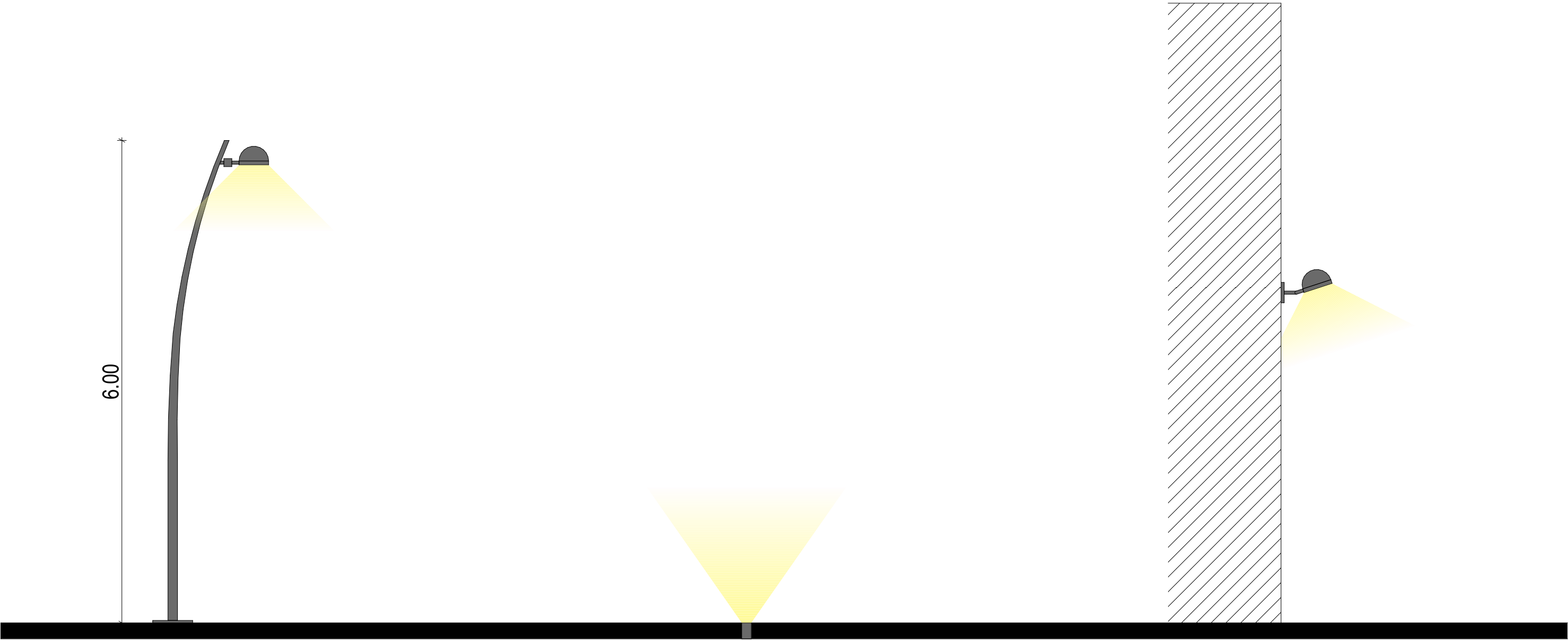
IGUZZINI ARGO BP 29 / GREY 15 / WARM WHITE / 60,4 W SHAPED POLES / CURVED CONICAL 1506 / WITH PLATE / H= 6000
